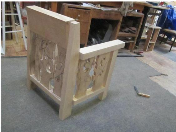
These two photos show you more about how the chair is constructed. One is a side of the chair disassembled, the other is the chair back. You can see the mortise and tenon joinery everywhere, and the angled joinery on the arm giving it a gentle slope for comfort.
