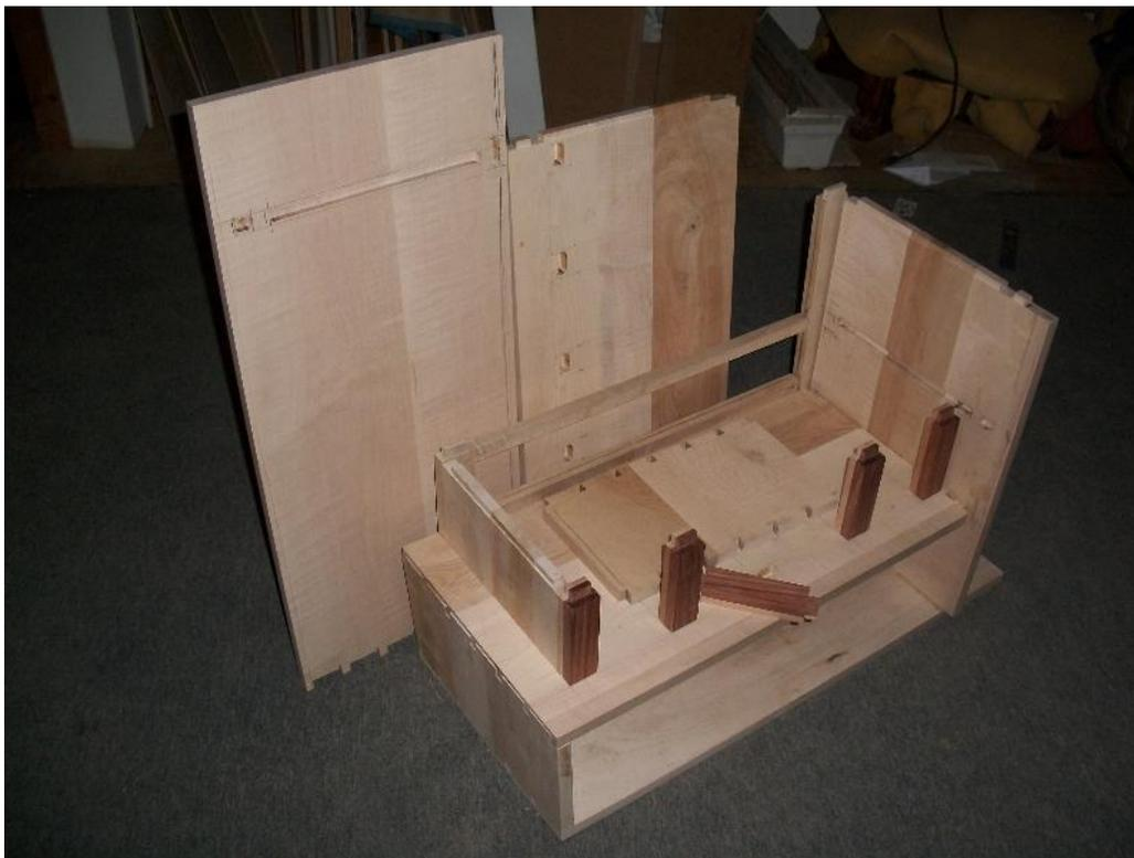
I've made this photo bigger so you can see the joinery. The bottoms of the side cabinets are with dovetails and you can see one setting in the middle. You can see the mortise and
