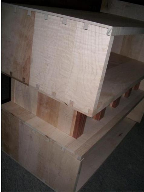
Here's a view of the dovetails on the bottom, which you won't be able to see when it's set up. So why bother? Because it's strong. I've drawn a small diagonal line on the corner at the top of the page. The door will be a full overlay door, but I have an idea to minimize how it is seen from the side by a sort of mitered configuration. I've got a hinge that I believe will work for this, and I'm making a test fit to make sure before cutting into the cabinet stock. More on this later.
