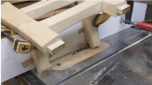
Cutting the tenons on the bracing below the right bench two at once by clamping the partially assembled structure to a box that slides on my table saw fence, and the cut tenons with the long brace. The base is setting on top of the seat to show the configuration, but you may need to look at the models from a past newsletter to really understand this photo.
