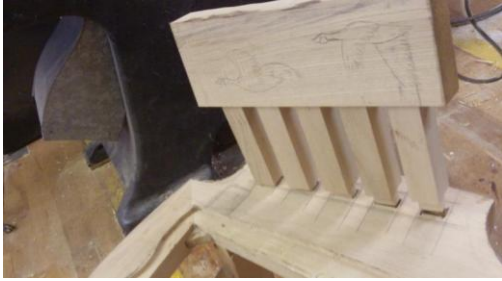
The seat back showing the five uprights, in a Nakashima style, and the legs and bracing on the underside of the right bench
