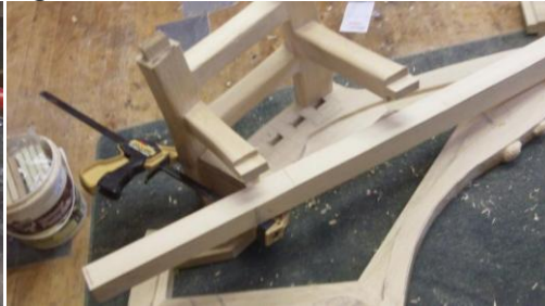
Cutting the tenons on the bracing below the right bench two at once by clamping the partially assembled structure to a box that slides on my table saw fence, and the cut tenons with the long brace. The base is setting on top of the seat to show the configuration, but you may need to look at the models from a past newsletter to really understand this photo.
