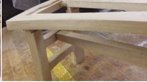
The seat back showing the five uprights, in a Nakashima style, and the legs and bracing on the underside of the right bench
